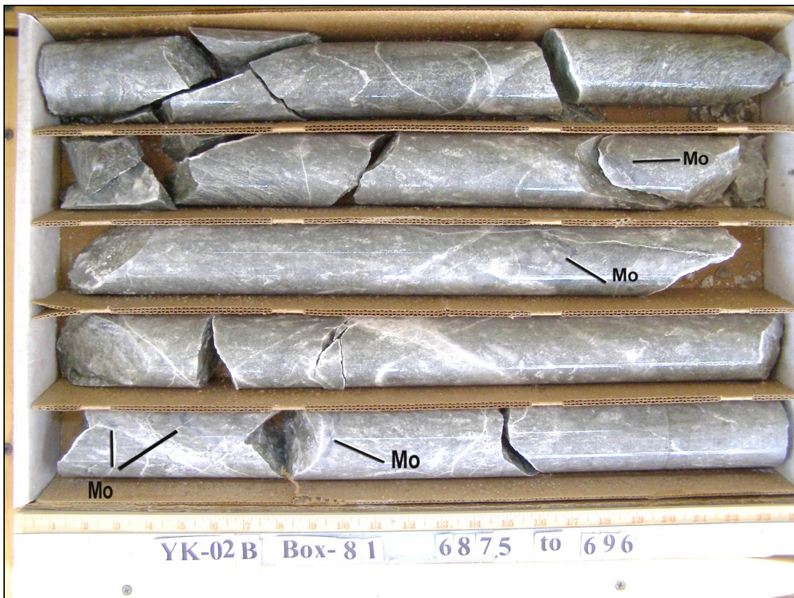
Figure 5-39. Stage 4 alaskitic aplo-granite-hosting molybdenum-copper mineralization
