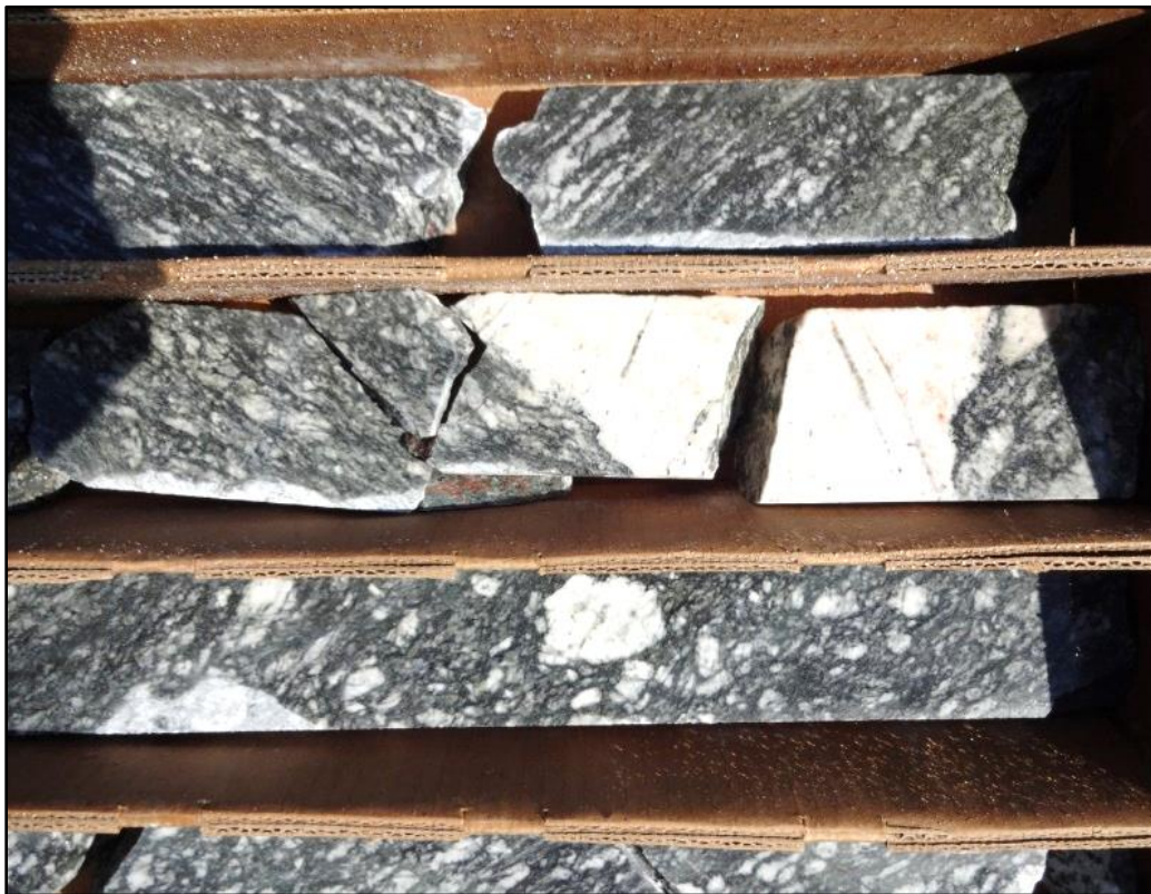
Figure 5-33 Porphyritic texture grading into schistose mylonitic deformation in the stage 3 monzonite to quartz monzonite intrusive phase
