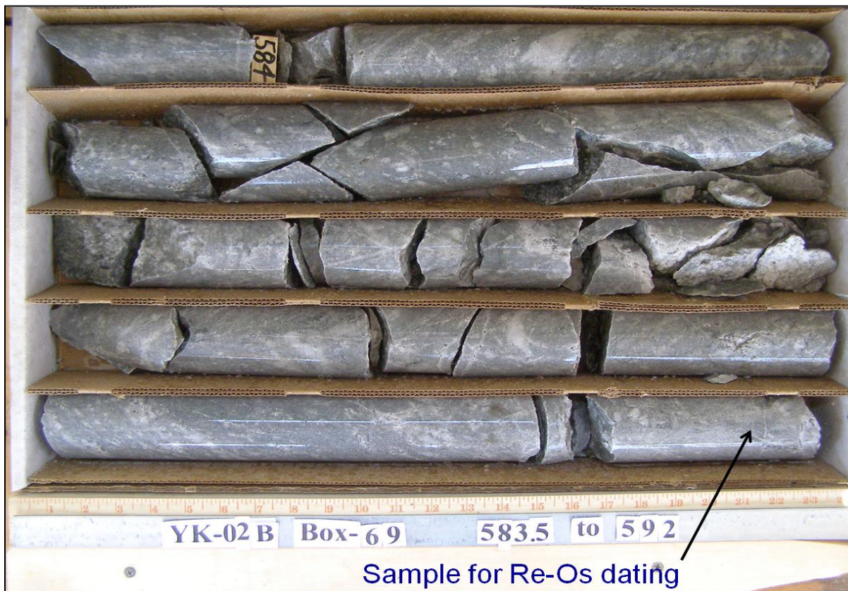
Figure 5-27 Alaskite-hosted molybdenite (chalcopyrite-pyrite) metallization in diamond drillhole YK-02B in the Yuma mine area showing location of age-date sample
