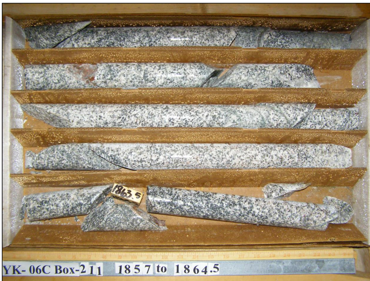
Figure 5-31. ‘Salt and pepper’ textured, medium-grained, hornblende (biotite) syenodiorite intrusion in drill YK-06c at 1857-1864 feet. The white parts of the core consist of albite alteration, which is a widespread propylitic alteration phase in the Stage 2 hornblende syenodiorite.
