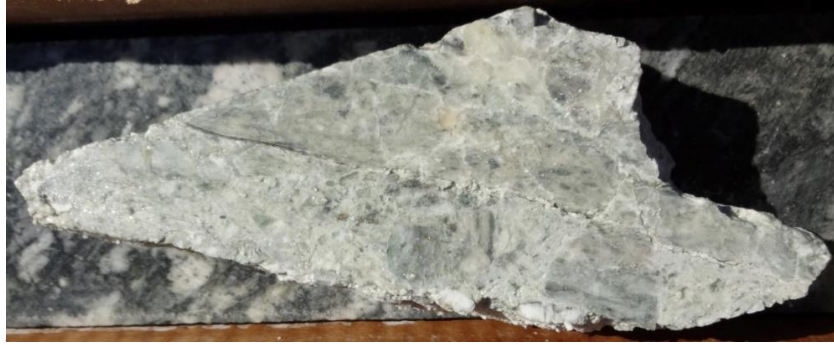
Figure 5-38. Intrusive breccia at contact of Stage 4 Mo-Cu alaskitic aplogranite and foliated biotite quartz monzonite porphyry at 980 feet in drillhole AZ11-1
