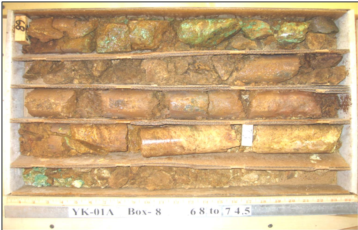
Figure 5-44 Copper oxide mineralization in YK01-A, 68 ft depth
