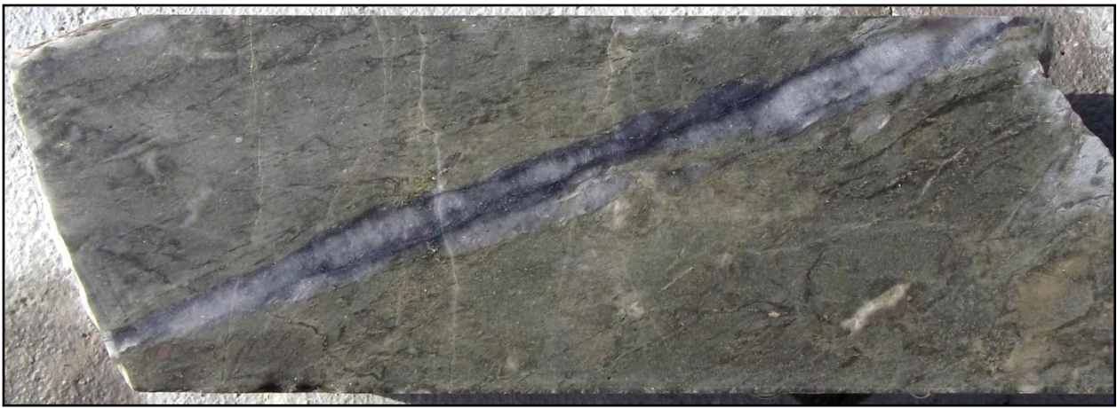
Figure 8-26 Quartz-(anhydrite-molybdenite-bearing vein in sheared diopside skarn about 30 ft above the copper-bearing skarn section at 1133 ft.
