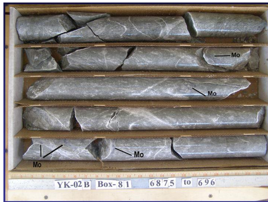
Figure 5-28 Mo-Cu mineralization associated of Stage 4, syenite/alaskite porphyry
