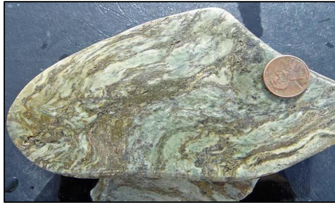
Figure 5-19 Chalcopyrite-pyrite-magnetite primary sulfide replacement mineralization (Stage 3) associated with quartz monzonite and overprinted by sillimanite in the center
