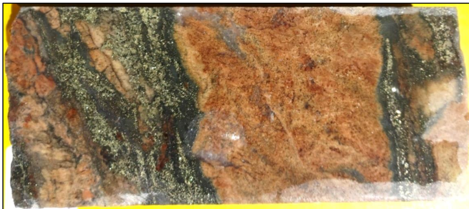
Figure 5-34. Net textured chalcopyrite-magnetite band within reddish andradite garnet at 1186 feet depth in drillhole AZ11-1. Core from this interval assayed 18,600 ppm Cu, 363 ppm Mo, 370 ppb Re, 220 ppb Au, and 19 ppm Ag.
