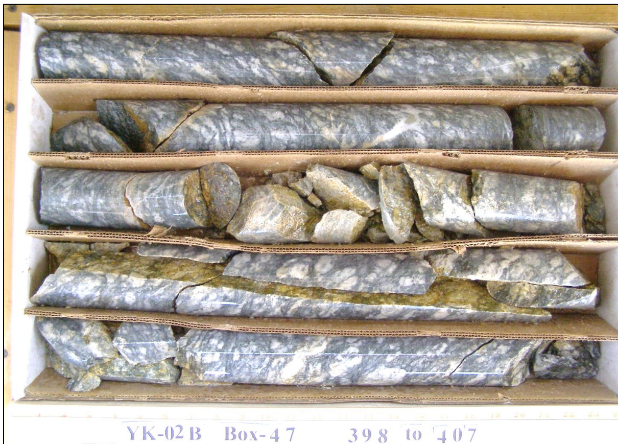
Figure 5-36. Stage 3 quartz monzonite porphyry-hosted copper-molybdenum mineralization
