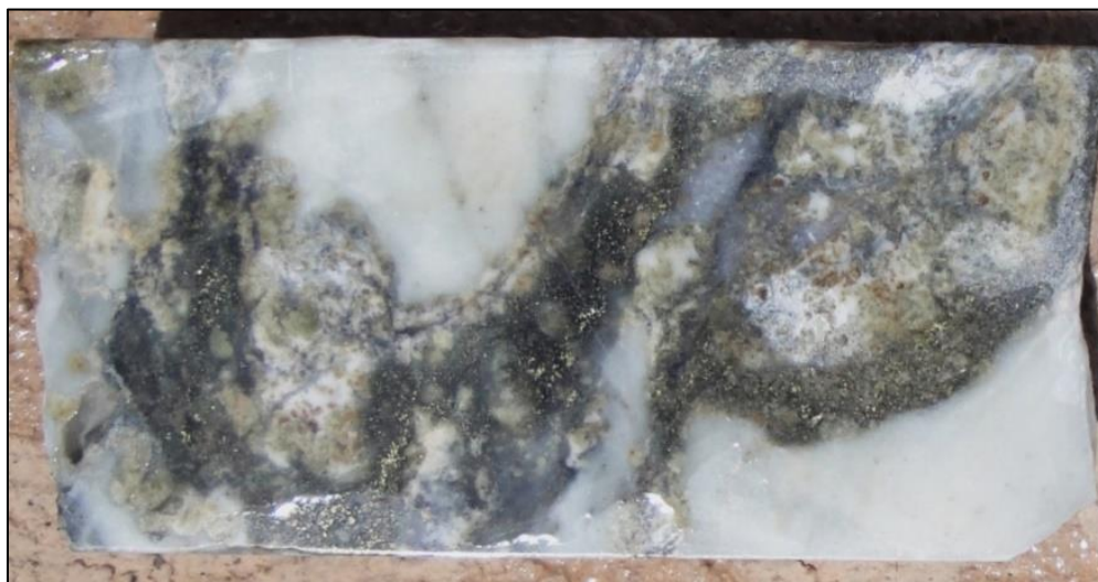
Figure 5-35. Deformed chalcopyrite-magnetite skarn with quartz veining folded into calcite-marble from 1193 feet in drillhole AZ11-1. Core from this interval assayed 3,170 ppm Cu, 53.2 ppm Mo, 31 ppm Re, 141 ppb Au, and 2.9 ppm Ag.
