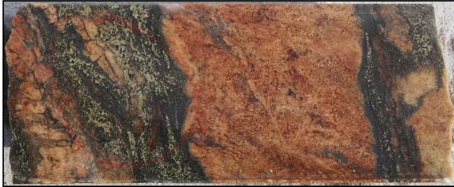
Figure 8-23 Highly metalized andradite-grossular garnet (pinkish red vitreous aggregates) with intervening magnetite-chalcopyrite layers from the 1190 ft depth in core from AV1-11
