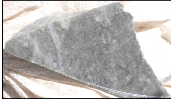
Figure 5-25 Molybdenite (gray line) and chalcopyrite (Stage 4) in Yuma King drill core
