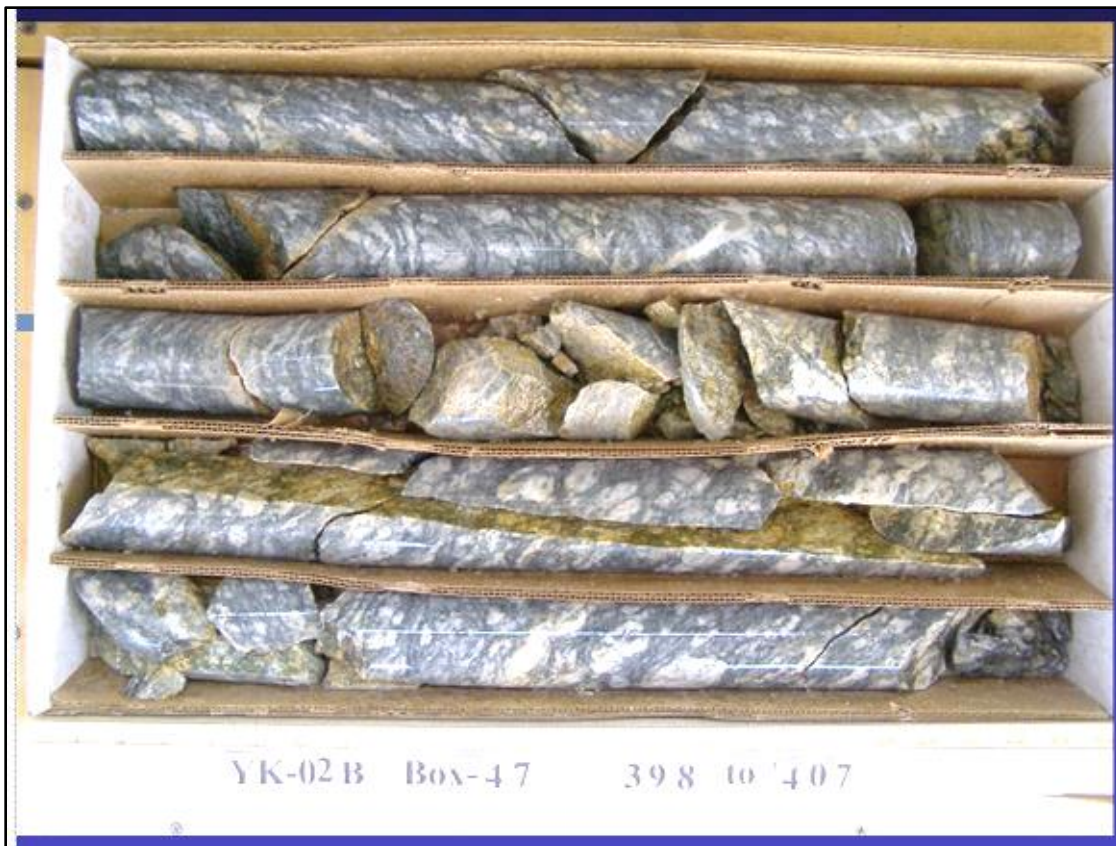
Figure 5-24 Core box showing drill intercept of copper-bearing monzonite porphyry in drill hole YK-02B that is host to most of the Cu-Mo mineralization at Yuma King
