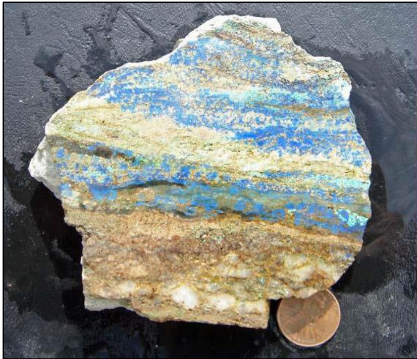
Figure 5-42 Azurite and malachite mineralization from the Yuma mine
