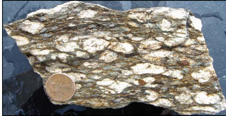
Figure 5-23 Sheared, chlorite-altered, quartz monzonite porphyry associated with Stage 3 copper-gold-molybdenum porphyry mineralization
